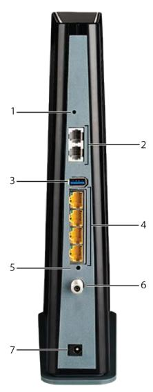
1. Connect one end of the coax cable to the cable outlet or splitter, and the other end to the Telephony Gateway's Cable connector (6). Tighten the connections by hand, then tighten an additional 1/8 turn with a wrench.
