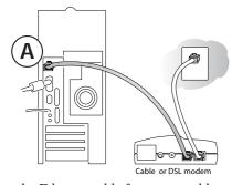
c. Connect the Ethernet cable from your cable or DSL modem to the Internet port (A) on the WGR614.
