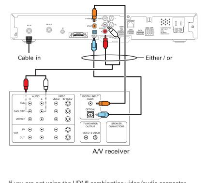
If you are not using the HDMI combination video/audio connector, the optical digital connector is the preferred audio connection if your entertainment system has it. Digital Coax input is next in the order of optimal performance. Stereo (red and white) connectors are the third choice and will not support Dolby Digital Surround sound.
